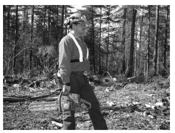
Carry the chain saw at your side with the bar pointing back and with the engine off or the chain brake set.
