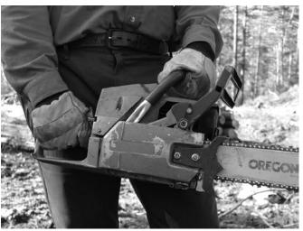
Hold the chain saw with two hands anytime it is running and the brake is not on. Keep the thumb of your left hand wrapped under the forward handle so that the saw cannot easily be pushed back out of your grasp.
