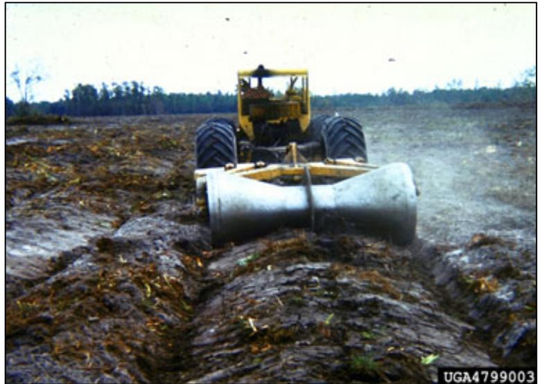
**EQUIPMENT:** Use a bulldozer of D-6 size or larger and a bedding machine capable creating a bed 18 inches deep x 30 inches wide. In a clean field, a farm tractor and bottom plow may be used to build smaller, less uniform beds.
