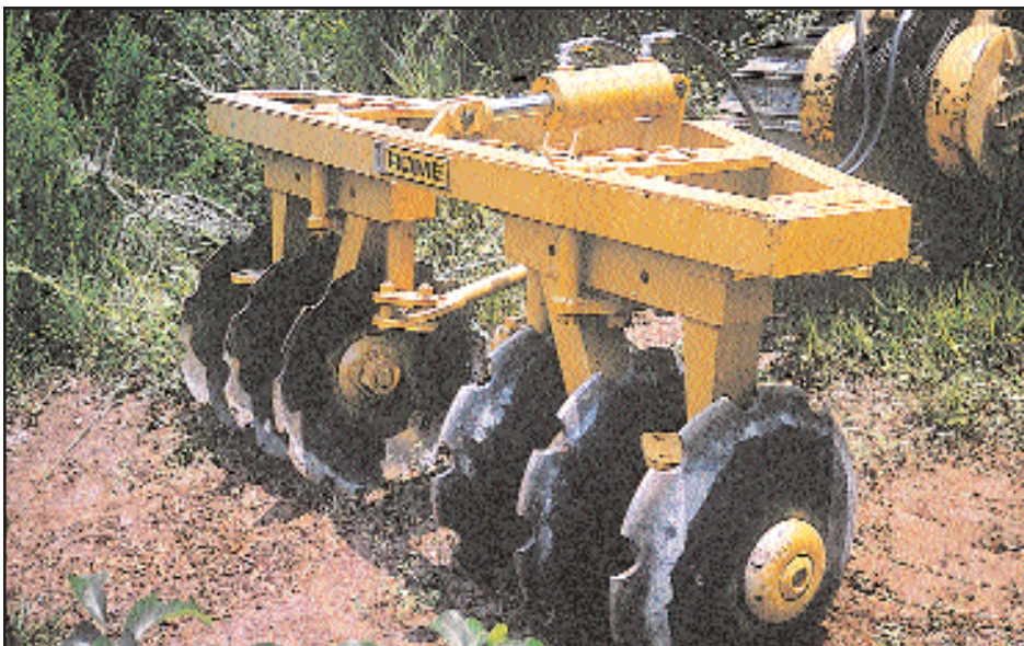
Disking is a good method if the terrain will allow the large areas of exposed soil without eroding.
