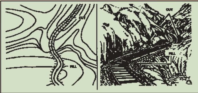
Figure 15 - Cut and fill.
