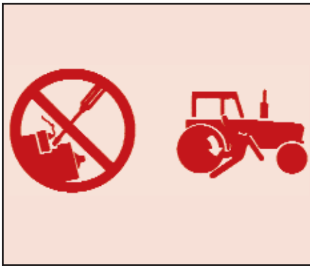
Figure 2 - Never attempt to start the engine by shorting across the starter terminals.
