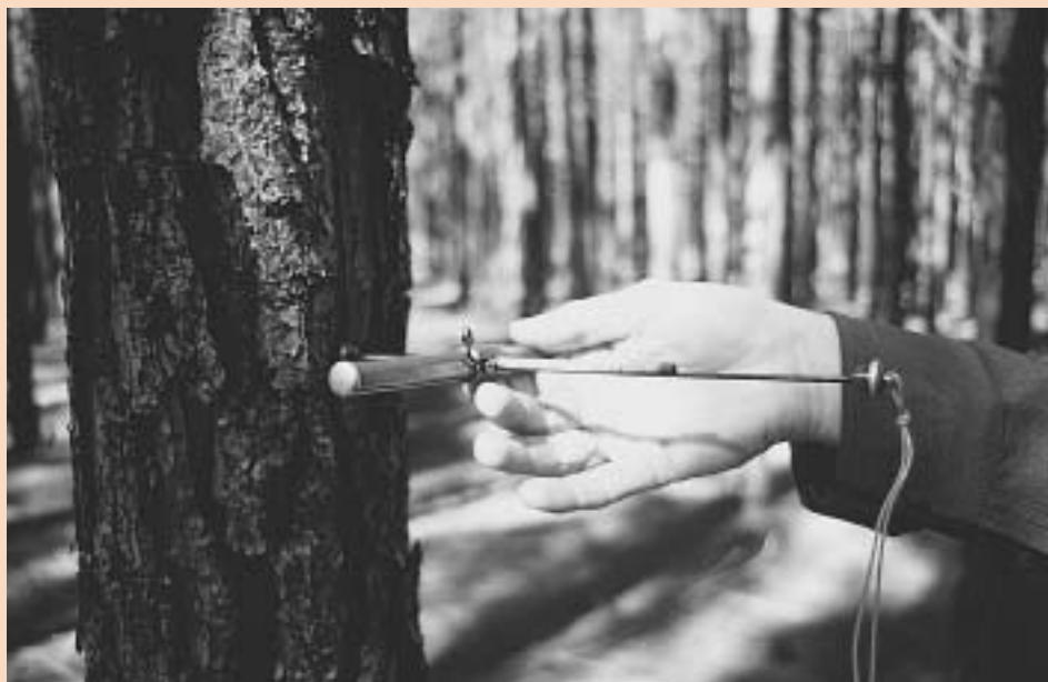
The approximate age of a tree can be determined with an increment borer.
